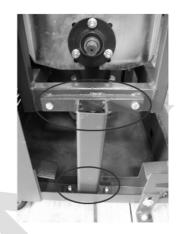
Use Spanner no. 13 to remove the Hex bolts (4 bolts each side).
