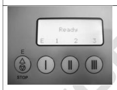
Unclamp the top plate to the fullest as per Can size by keep pressing button "E"
