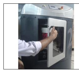
Once the cycle completes, the gyro will be automatically moved to vertical position & will stop. The clamping jaw will get released and the door will get unlock. Open the door & press the Can tray locking lever up and pull the tray outward. Remove the Can from bottom disc. Press the Can tray locking lever up and slide the tray inside.
