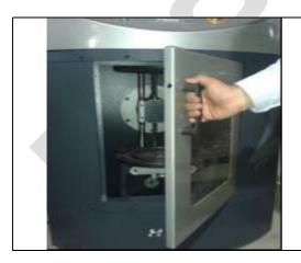
Open the Mixer door to its fully open position.
