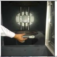
Unlock the Clamping Jaws by pressing button 'E' as per the Can size.
