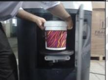
Place the Can which is to be mixed on the bottom disc.
