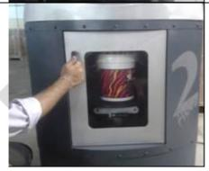
Close the door (The door has to be closed in order to start the mixing cycle).
