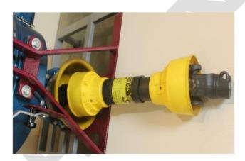
Connect the drive shaft to the PTO of the duster ensuring that the locking pin in the shaft is positioned in the appropriate cavity finally attach the safety chains provided to the shaft
